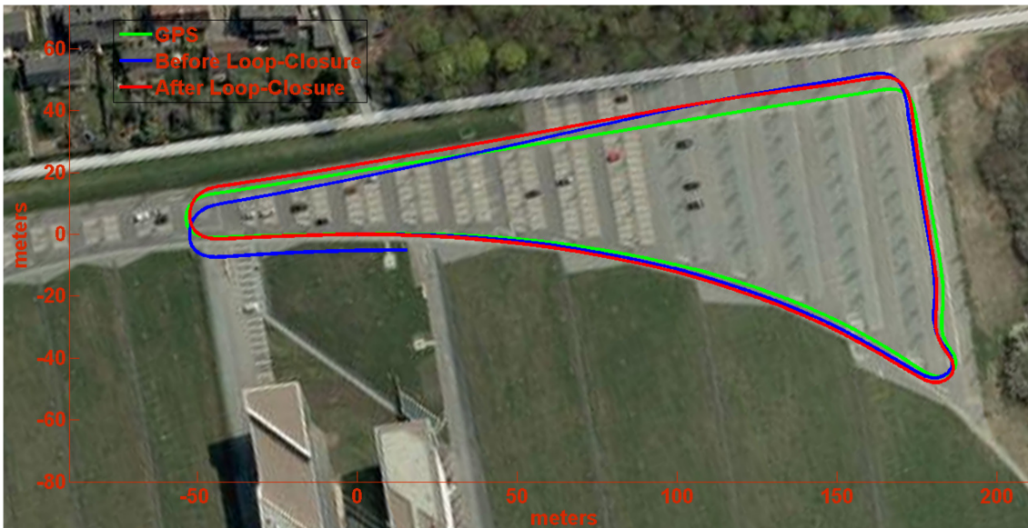
Figure 7: Top view of the recovered trajectory with enhancements compared to the GPS/INS ground truth. (Source: [1])
